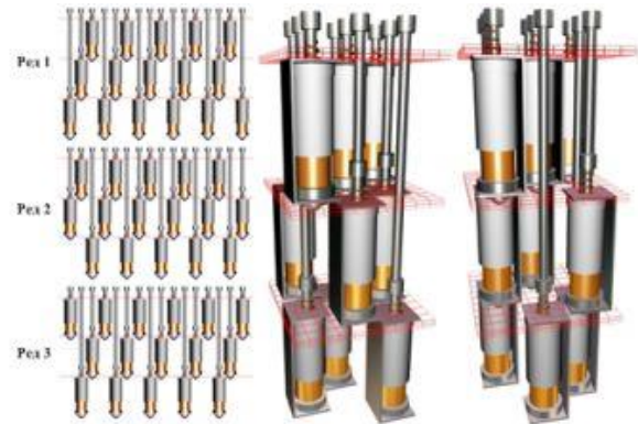
Fig. 4. Arrangement of solenoids by rows and columns
